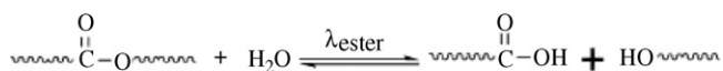
Scheme 4. The proposed hydrolytic degradation process of polyesters. Reproduced from Qian et al. (2004), with permission.
